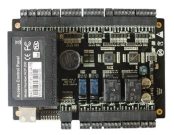
RFID access control panel - Access with card or password - TCP/IP communication | RS485 - 4 Wiegand readers - Relay output for 2 doors - ZKBioAccess
