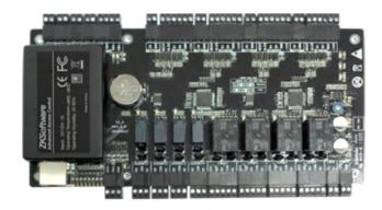
RFID access control panel - Access with card or password - TCP/IP communication | RS485 - 4 Wiegand readers - Relay output for 4 doors - ZKBioAccess
