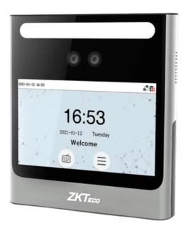
Access control - Facial, PIN and EM card - 4.3" TFT touch screen - 500 faces | 150.000 records - TCP/IP, WiFi and USB - ZKBioAccess software 5 doors included
