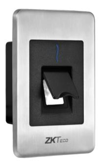
Access reader - Silk ID fingerprint and EM card access - LED and acoustic indicator - RS485 - Compatible with ZK-ATLAS-x60 - Embedded installation | Suitable for outdoor use
