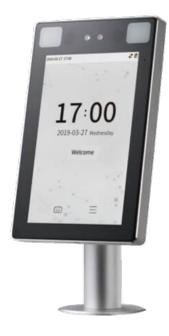
Access and presence control for turnstiles - Facial, Palm, EM card and PIN - 30.000 faces | 1.000.000 records - Display 8" IPS touch screen | TCP/IP & WiFi - Suitable for outdoor use IP68 | Vandal resistant IK04 - ZKBioTime8/ ZKBioCVSecurity/ZKGoTimeCloud
