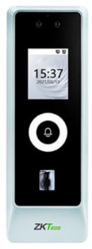
Access control - Facial, fingerprint and EM/MF card - 10.000 fingerprints | 500.000 records - Display 2" TFT | TCP/IP, RS485, Wiegand and relay - Suitable for outdoor use IP66 | Vandal resistant IK07 - Softwares ZKBioAccess / ZKBio CVSecurity
