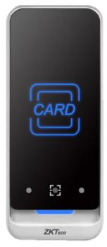
Access reader - QR code and EM card access - LED and acoustic indicator - Wiegand 26/34 | RS485 - Compatible with ZKTeco controllers - Suitable for exterior IP65
