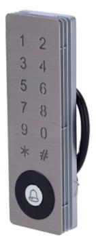
Access control and access reader - MF Card and PIN - 5.000 cards | 5.000 users - Integrated controller | Wiegand 26/34 - Compatible with ZKTeco controllers - Suitable for outdoor use IP65 | Anti-vandalism
