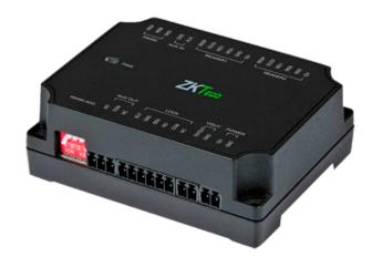
Extending Access Controller - Access with card or password - RS485 Communication - 2 Wiegand readers - Relay output for 1 door - Master controller ZK-C2-260 required
