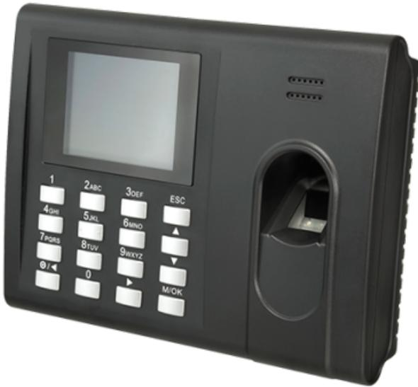
Simple Time & Attendance and Access control - Fingerprint, EM card and PIN - 3.000 fingerprints | 50.000 records - TCP/IP, USB and relay - Time & Attendance control mode management - ZKBioTime software 8 2 devices included
