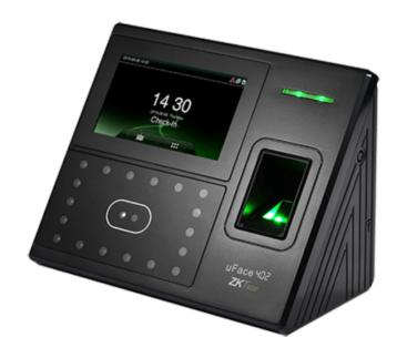
Time & Attendance and Access control - Fingerprints, EM RFID Card, facial and keypad - 4000 recordings / 100.000 records - TCP/IP, USB and Relay - Time & Attendance control mode management - ZKBioTime software 8 2 devices included
