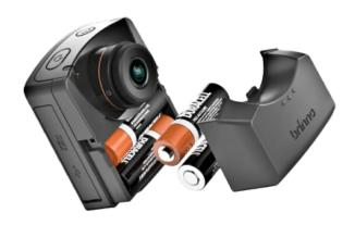
Brinno Time Lapse Camera - Resolution 1080p Full HD - 2" TFT LCD display - SD card recording up to 128GB - Battery powered - Includes IP65 housing and bracket
