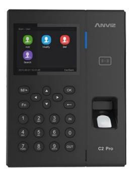
Time & Attendance and Access control - Fingerprints, MF and keyboard - 5000 recordings / 100000 records - WiFi, TCP/IP, USB, RS232, Relay - 8 Time & Attendance control modes - CrossChex and Cloudclocking Software
