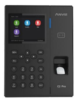
PoE Time & Attendance and Access control - Fingerprints, RFID EM and keypad - 10000 recordings / 100000 records - WiFi, TCP/IP, USB, integrated controller - 8 Time & Attendance control modes - Anviz CrossChex Software
