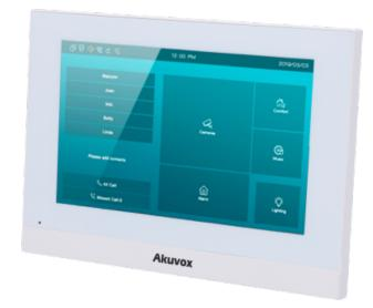
Linux Monitor for Video Door Station - 7" TFT Screen - Crystal Clear two-way audio - TCP/IP, PoE, WiFi, Standard SIP - Cloud-based maintenance - Connection of monitor and boards via Cloud
