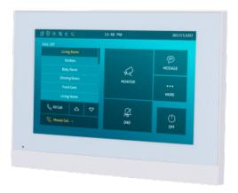
Android 6.0 monitor for Video Door Station - TFT display of 7" | Third-party applications - Crystal Clear two-way audio - TCP/IP, PoE, WiFi, Bluetooth, SIP Standard - Cloud-based maintenance - Connection of monitor and boards via Cloud
