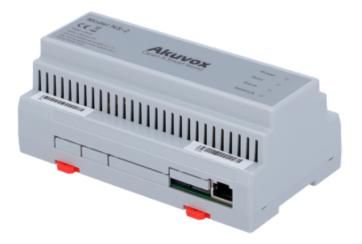
2-wire to IP converter - 6 groups of 2-hilos - TCP/IP with RJ45 - Powers 2-hilos devices - Connection of cascade converters - DIN rail mount
