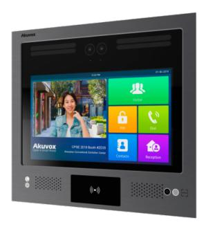
Vandal-resistant surface IP video door entry system - Dual camera 2 Mpx | Bidirectional audio and video - Facial, card, PIN and QR | 4 relays - Apartments : PoE+, LTE, standard SIP - IPS 13" touchscreen | Cloud Maintenance - Connection via Cloud | Output 12V
