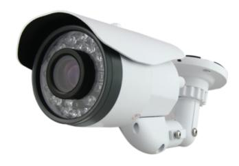
HDTVI, HDCVI, AHD and Analogue camera - 1080p (25 fps) - 1/2.9" Sony© 2.19 Mpix Exmor - 5~50 mm Varifocal lens - 6 LEDs Array Range 100 m - Remote OSD menu
