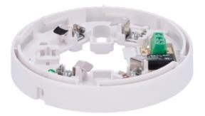
Low profile base with relay - Up to 12VDC 0.5A / Terminal NO/NC/C - Compatible with V2 and high-base detectors - Necessary for the detector installation - Easy mounting mark - Possibility of locking the detector to the base - Compatible with action indicator light
