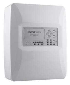
2 Zone Conventional Fire Alarm Panel - 2 Siren output - 2 alarm and fault outputs and 2 configurable relay outputs - Repeater output - Up to 30 detectors per zone - End-of-line resistance auto detection
