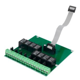
DMTECH Conventional Relay Module - 8 relay outputs - Up to 3A/125VAC or 3A/30VDC - Centrally powered - Compatible with DMTECH fire panels
