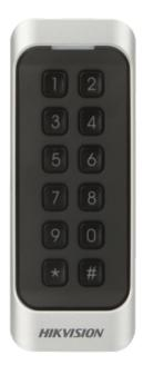
Access reader for frames - Access by MF card and PIN - LED and acoustic indicator - Wiegand 26/34 | RS485 - Compatible with Hikvision controllers - Suitable for exterior IP65
