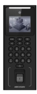
Access Control and Time & Attendance - Facial, fingerprint, EM card and PIN - 500 users | 150.000 records - TCP/IP, USB and RS485 - Integrated controller (sensor, pushbutton and relay) - iVMS-4200 | Hik-Connect
