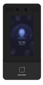
Access Control and Time & Attendance - Face, EM card, QR and PIN - 1.500 users | 150.000 records - TCP/IP, WiFi, USB, RS485 and Wiegand | IP65 - Integrated controller (sensor, pushbutton and relay) - iVMS-4200 | Hik-Connect
