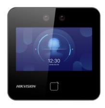
Access Control and Time & Attendance - Facial, MF card and PIN - 1.500 users | 150.000 records - TCP/IP, WiFi, USB, RS485 and Wiegand - Integrated controller (sensor, pushbutton and relay) - iVMS-4200 | Hik-Connect
