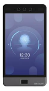
Access Control and Time & Attendance - Facial, fingerprint, iris, MF-card and PIN - 5.000 users | 150.000 records - TCP/IP, WiFi, USB, RS485 and Wiegand | IP65 - Integrated controller (sensor, pushbutton and relay) - iVMS-4200 | Hik-Connect
