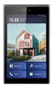
Android WiFi IP video door phone for apartments - 2 MP Camera | Bidirectional Audio - Facial, MF card, QR and PIN | 2 relays - Mobile App via monitor - IPS 10" touch screen 500 apartments - Surface or recessed mounting | IP65
