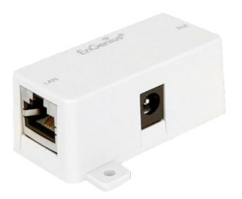
PoE injector - Data and power on a single UTP cable - Input RJ45 / DC IN - Output RJ45 (PoE and Data) - Max Power 15.4 W / DC 24 V - EnGenius PoE specific antennas
