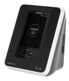
ANVIZ Access Control and Time & Attendance - Biometric facial system with dual sensor - Facial recognition, card and PIN - 3.000 users | 100.000 records - 8 presence modes | Integrated controller - CrossChex software
